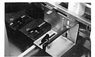
Quick turn Kipp handles make carton changeover fast and accurate.
